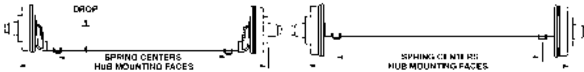
Difference Between Hub Face and Spring Center
