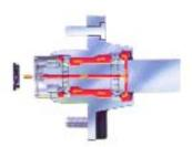
With such complete lubrication, your running gear is protected from corrosion and water entry. E-Z Lube protection and maintenance features make it ideal for almost any towable axle, whether it's for work or play.
